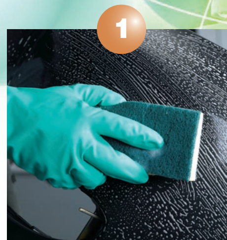
Clean and Scuff
