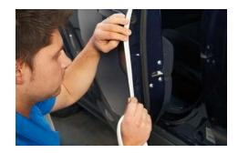
For a moving part, apply to the panel edge making sure the adhesive is behind the panel. Press evenly and firmly for good adhesion.
