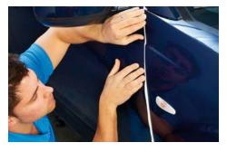
Close the part carefully to make sure the foam is exposed then smooth the tape into the gap with your finger to the required depth.
