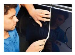
Close the moving part very carefully and then do a visual check to make sure there is no exposed adhesive.
