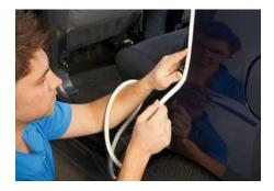
Apply to the car body / fixed part being careful not to expose the adhesive where paint will be applied. Press evenly and firmly for good adhesion.
