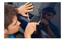
A spreader can also be used to adjust the height or depth of the premium foam masking tape to ensure perfect coverage.
