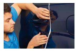
Close the part and smooth the foam tape into the gap with your finger to the required depth.
